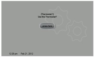
After power is applied to the thermostat for the first time, it displays the iComfort® "splash screen", checks the system for installed communicating devices, and displays the "Use this thermostat?" screen.
