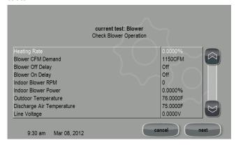
When a test is running, a status screen will show which test is being run and the results. Use the up / down arrows to scroll through the results.
