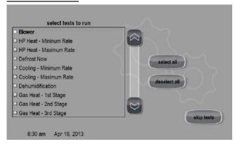
A variety of system tests can be performed by the installer. Select the tests to be performed individually by touching the checkboxes or use the Select All Button to run all available tests. Use the Deselect All Button to uncheck all boxes.
