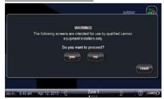
When the Home Screen is displayed touch and hold the **LENNOX** Logo Button for 5-6 seconds to switch to the Installer Mode Screen.
