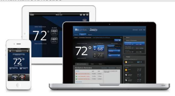
Wi-Fi remote temperature monitoring and adjustment through a home wireless network via desktop PCs, laptops, and apps for smartphones or tablets.
